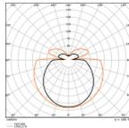
Scheda tecnica Ledvance Tubo LED T8 EM Ultra Output Value Conventional (EM), Mains (AC) Ultra Output 29W 3500lm - 840 Bianco Freddo | 150cm - Sostitutiva 58W
