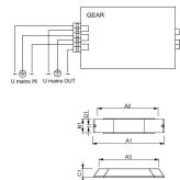
Scheda tecnica Philips HID-PV m 20 / I CDM HPF 220-240V 50/60Hz
